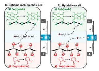
Scheme 1 Schematic of the working principle of the PI-PC full-cell during the discharge process in a cationic rocking-chair mode with Li<sup>+</sup>,  $Zn^{2+}$  or  $Al^{3+}$  (a), and hybrid-ion configuration with  $Li^+/H^+$  (b).
