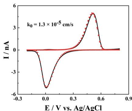
Fig. 6 The cyclic voltammograms of 1 mM  $\text{FeCl}_3$  in 0.5 M  $\text{H}_2\text{SO}_4$  and 0.1 M KCl from the simulation (red points) and experiments (black solid line).  $a = 100 \text{ nm}$ .  $d = 1320a$ ,  $\tan \theta = 0.2$ ,  $v = 0.1 \text{ V s}^{-1}$ ,  $E_0 = 0.26 \text{ V}$  and  $k_0 = 1.3 \times 10^{-5} \text{ cm s}^{-1}$ .
