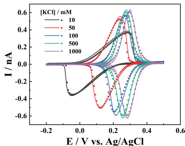
Fig. 5 Experimental (solid lines) and simulated (points)  $i$ - $V$  curves for different concentrations of KCl ( $c_1$ ). The  $K_4Fe(CN)_6$  concentration is  $1$  mM.  $c_1$ , mM:  $10$ ,  $50$ ,  $100$ ,  $500$ , and  $1000$ .  $a = 50$  nm,  $d = 1100a$ ,  $\tan \theta = 0.19$ ,  $v = 0.1$  V  $s^{-1}$  and  $E_0$  is  $0.12$ ,  $0.18$ ,  $0.24$ ,  $0.265$ , and  $0.29$  V.
