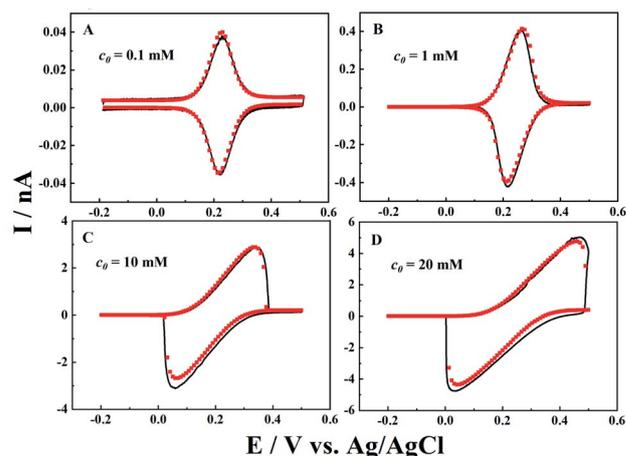
Fig. 4 Experimental (black solid lines) and simulated (red points)  $i$ - $V$  curves for different concentrations of  $K_4Fe(CN)_6$  ( $c_0$ ). The background solution is  $0.1$  M KCl.  $a = 50$  nm,  $d = 1000a$ ,  $\tan \theta = 0.2$ ,  $v = 0.1$  V  $s^{-1}$  and  $E_0 = 0.21$  V,  $0.24$  V,  $0.2$  V, and  $0.25$  V.
