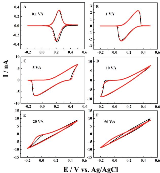
Fig. 2 Effect of scan rate on  $i$ - $V$  curves in 1 mM  $K_4Fe(CN)_6$  + 0.1 M KCl. From panels (A) to (F), the experimental (black solid lines) and simulated (red points)  $i$ - $V$  curves are at scan rates of 0.1, 1, 5, 10, 20, and 50 V  $s^{-1}$ . Fitting parameters:  $a = 50$  nm,  $d = 2000a$ ,  $\tan \theta = 0.2$  and  $E^0 = 0.21$  V.
