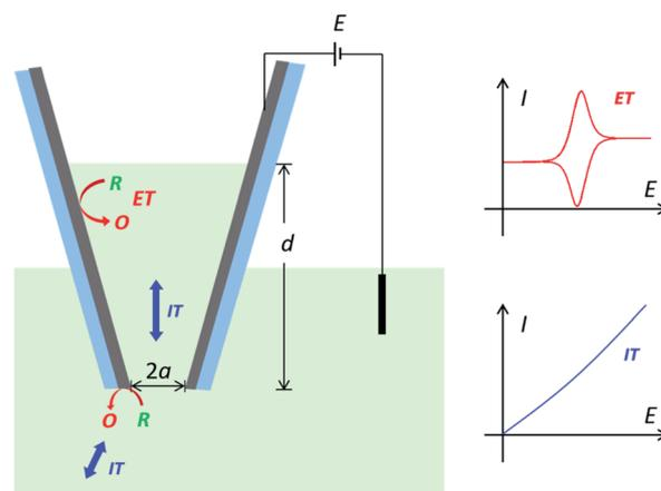
**Scheme 1** The charge transport processes in carbon nanopipettes. When applying a potential at the carbon layer, the measured current signal would be determined by both the ion transport processes in the nanopipette and the electron transfer processes at the carbon layer.
