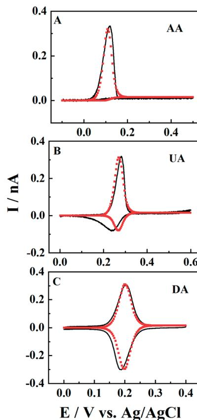
Fig. 7 The experimental (black solid lines) and simulated (red points) voltammograms of AA, UA and DA in CNPs. The concentration is 0.5 mM with 10 mM PBS (pH 7.4) buffer. Fitted value:  $a = 50 \text{ nm}$ ,  $d = 800a$ ,  $\tan \theta = 0.15$ , and  $v = 0.1 \text{ V s}^{-1}$ .  $k_c > 0.8$ ,  $k_c = 0.2$ , and  $k_c < 0.01 \text{ s}^{-1}$  and  $E_0 = 0.11/0.27/0.2 \text{ V}$  for AA, UA and DA.
