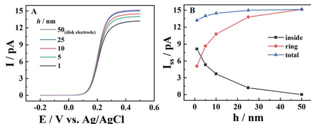
Fig. 1 The simulated steady-state voltammograms of CNPs with different thicknesses ( $h$ ) of deposited carbon. The solution is 1 mM  $K_4Fe(CN)_6$  + 0.1 M KCl.  $a = (50 - h)$  nm,  $d = 400a$ ,  $\tan \theta = 0.2$ ,  $v = 0.1$  V  $s^{-1}$  and  $E^0 = 0.2$  V vs. Ag/AgCl.
