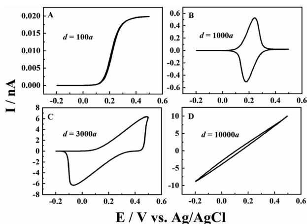
Fig. 3 Simulated  $i$ - $V$  responses from a CNP at different solution depths in  $1$  mM  $K_4Fe(CN)_6$  +  $0.1$  M KCl. From panels (A) to (D), the solution depth is  $100a$ ,  $1000a$ ,  $3000a$ , and  $10\,000a$ .  $a = 50$  nm,  $\tan \theta = 0.2$ ,  $v = 0.1$  V  $s^{-1}$  and  $E^0 = 0.2$  V.
