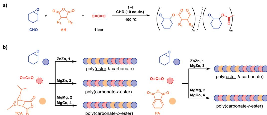
**Scheme 1** (a) Schematic showing the synthesis of different copolymers from mixtures of cyclohexene oxide (CHO), anhydride (AH), and CO<sub>2</sub>, with catalysts 1–4. (b) Summary of catalyst selectivity and the resulting polymer architectures. Note that changing from CO<sub>2</sub> to N<sub>2</sub> atmosphere is required when using catalysts 2 and 4 to ensure ester formation.
