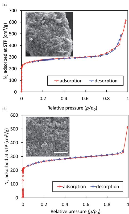
**Fig. 5** BET adsorption plots for: (A) Li-BIF-3, showing a surface area of  $1010 \text{ m}^2 \text{g}^{-1}$  and (B) Cu-BIF-3, showing a surface area of  $935 \text{ m}^2 \text{g}^{-1}$ . The insets in (A) and (B) are representative SEM images of the mechanochemically prepared BIF samples, with scale bars corresponding to  $4 \mu\text{m}$  and  $5 \mu\text{m}$  shown in white.
