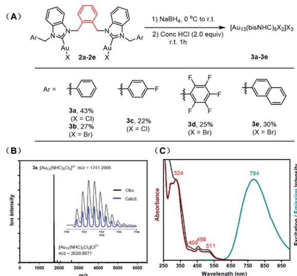
Fig. 2 (A) Preparation of [Au<sub>13</sub>(bisNHC)<sub>5</sub>X<sub>2</sub>]<sub>3</sub> nanoclusters [3a–e]<sub>3</sub> (B) ESI-MS of [3a]Cl<sub>3</sub>; (C) UV-vis absorbance (red), photoluminescence excitation (black) and emission (green) spectra of [3a]Cl<sub>3</sub> in dichloromethane.
