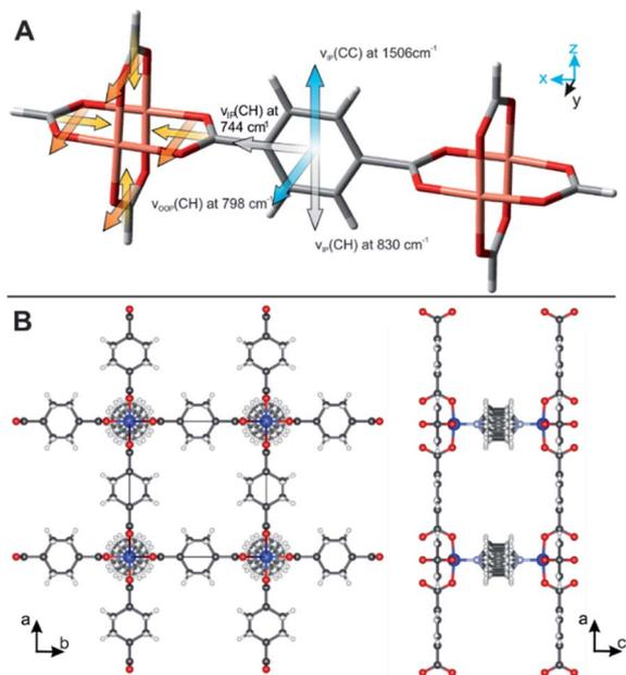
Fig. 7 (A) Illustration of the transition dipole moments for the aromatic vibrations found in the BDC linker. (B) Crystal structure of  $\text{Cu}_2(\text{BDC})_2\text{DABCO}$  with the proposed aromatic linker orientation perpendicular to the carboxylate plane.
