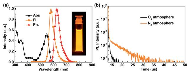
Fig. 2 (a) Absorption spectrum (Abs.), fluorescence spectrum (Fl.), and phosphorescence spectrum (Ph.) of CNCz-BNCz in toluene solution at  $1 \times 10^{-5}$  mol L $^{-1}$  under ambient conditions. (b) Transient photoluminescence spectra of CNCz-BNCz in toluene solution at  $1 \times 10^{-5}$  mol L $^{-1}$  under an O $_2$  atmosphere and N $_2$  atmosphere, respectively.
