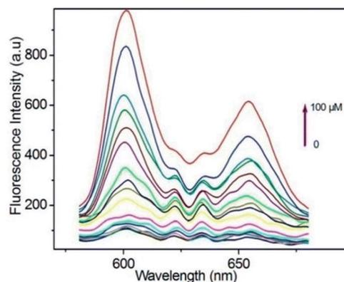
Fig. 14 Fluorescence spectra of porphyrin ligand ( $10 \mu\text{M}$ ) in BBS buffer (pH = 7.40, 20 mM) after titration with  $\text{HS}^-$  from 0–100  $\mu\text{M}$ ,  $\lambda_{\text{ex}} = 419$ . Reprinted with permission from ref. 94. Copyright (2014) American Chemical Society.
