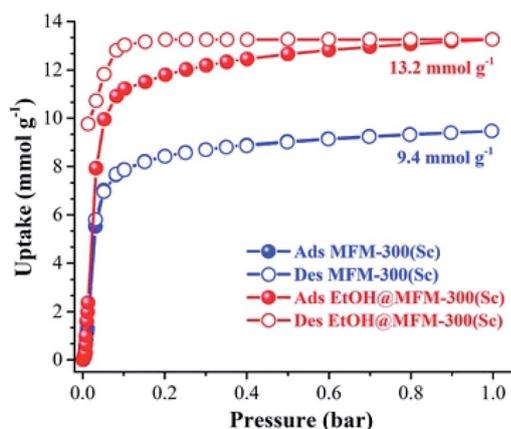
Fig. 4  $\text{SO}_2$  adsorption isotherm of scandium-based MFM-300 (blue isotherm) and after confinement of 2.8% EtOH (red isotherm). Reprinted with permission from ref. 37c. Published (2019) by The Royal Society of Chemistry.
