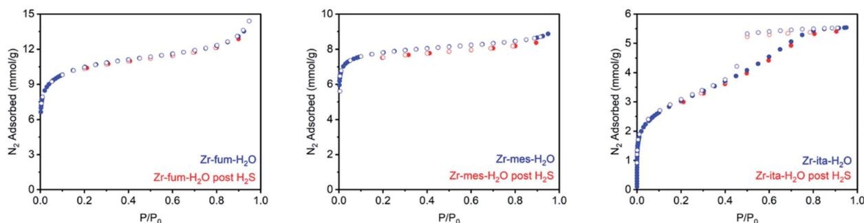
Fig. 5 77 K N<sub>2</sub> adsorption isotherms of activated Zr-fum-H<sub>2</sub>O, Zr-mes-H<sub>2</sub>O, and Zr-ita-H<sub>2</sub>O before (blue) and after treatment with H<sub>2</sub>S at 25 °C (red). After H<sub>2</sub>S adsorption, the MOFs were regenerated at 100 °C under vacuum (<10 μbar) for 48 h.
