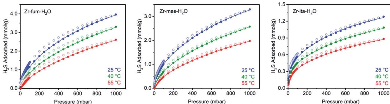
Fig. 3 H<sub>2</sub>S adsorption (closed circles) and desorption (open circles) isotherms at 25 °C (blue), 40 °C (green), and 55 °C (red) of activated Zr-fum-H<sub>2</sub>O, Zr-mes-H<sub>2</sub>O, and Zr-ita-H<sub>2</sub>O. Solid lines represent fits of the adsorption data to a Langmuir–Freundlich model. A data point was considered equilibrated after <0.01% pressure change occurred over a 45 s interval.
