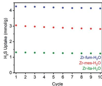
Fig. 6 Cycling capacities for H<sub>2</sub>S adsorption (1 bar, 30 °C) in Zr-fum-H<sub>2</sub>O, Zr-mes-H<sub>2</sub>O, and Zr-ita-H<sub>2</sub>O. The samples were regenerated at 100 °C under high vacuum (<10 μbar) between cycles.
