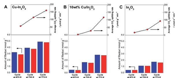
Fig. 4 Dependence of RWGS-CL performance of each oxide on the reaction temperature. Amounts of redox and average CO<sub>2</sub> splitting rate during the re-oxidation step on Cu–In<sub>2</sub>O<sub>3</sub> (A), 10 wt% Cu/In<sub>2</sub>O<sub>3</sub> (B), and In<sub>2</sub>O<sub>3</sub> (C). Reduction was conducted in a 10% H<sub>2</sub> atmosphere for 30 min; oxidation was conducted in a 10% CO<sub>2</sub> atmosphere.
