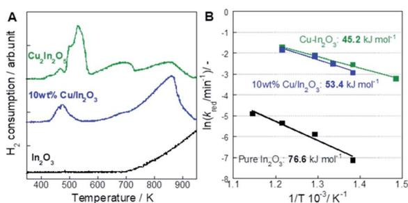
Fig. 5 Kinetics analysis of each oxide in the reduction step. (A) H<sub>2</sub>-TPR profiles for Cu–In<sub>2</sub>O<sub>3</sub> (derived from Cu<sub>2</sub>In<sub>2</sub>O<sub>5</sub>), 10 wt% Cu/In<sub>2</sub>O<sub>3</sub> and In<sub>2</sub>O<sub>3</sub>. (B) Arrhenius plots for the reduction of Cu–In<sub>2</sub>O<sub>3</sub> (derived from Cu<sub>2</sub>In<sub>2</sub>O<sub>5</sub>), 10 wt% Cu/In<sub>2</sub>O<sub>3</sub> and In<sub>2</sub>O<sub>3</sub>.
