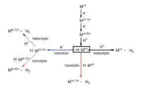
Fig. 13 Possible mechanisms for the hydrogen evolution reaction. Used with permission from ref. 2.
