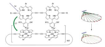
Fig. 3 As the porphyrin dimer becomes excited, energy transfer occurs to the ring with the same rate ( $\sim$ 1.3 ps) no matter its size (N=6, 8, 10, 12 or 30). A representation of the line-dipole model on the right shows the effect of strain induced by coordination. The transferred excitation is delocalized over 6 porphyrins. Adapted with permission from ref. 50.
