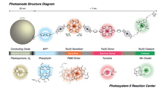
Fig. 36 The supramolecular layer-by-layer deposition using Zr-phosphonate chemistry preorganizes chromophores reminding of the PS II. The top system is fully artificial, but the components serve the same purpose those in the PS II Reaction Centre and transfer electrons over a large distance. Used with permission from ref. 141.
