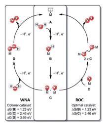
Fig. 7 Water oxidation catalysis follows either of two mechanisms. A mononuclear WNA mechanism or the binuclear ROC mechanism. Used with permission from ref. 69.
