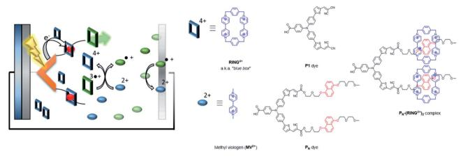
Fig. 32 Supramolecular interactions are implemented in p-type DSSC using the "blue box" as redox shuttle. The  $P_N$  dye is heterogenized onto NiO, and binds the ring prior to excitation. As soon as the ring is reduced, it loses affinity for the chromophore, dethreads and moves away while carrying the charge. Used with permission from ref. 129.
