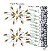
Fig. 31 Supramolecular antenna complexes are assembled onto ntype semi-conductors (TiO<sub>2</sub>) using hydrogen-bonding interactions. H<sub>2</sub>-porphyrin acceptor (blue discs) act as the seed for the growth of Zn-porphyrin antennae acting as energy donor. Used with permission from ref. 126
