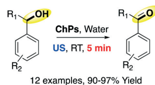
Scheme 18 Choline peroxydisulfate-promoted oxidation of benzyl alcohol derivatives to aldehydes in ultrasound. 67
