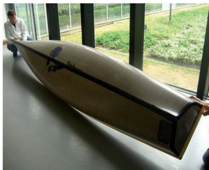
Fig. 2 Flax/PLA canoe manufactured during the NAVECOMAT project.
