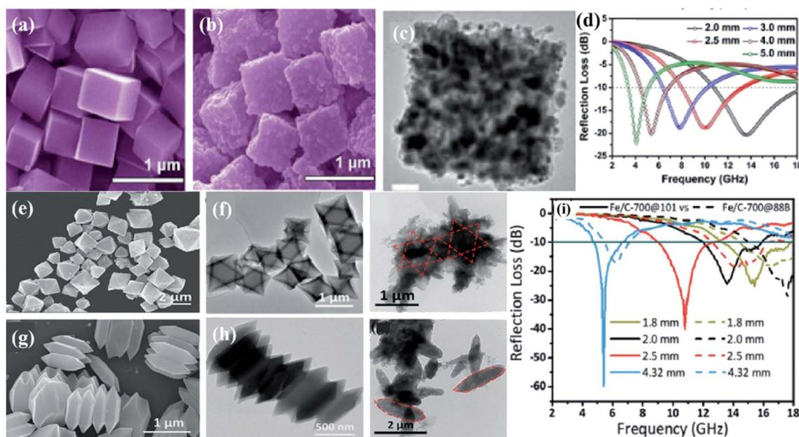
Fig. 4 SEM and TEM images of PB (a), Fe/C-PB (b and c), MIL-101-Fe (e), Fe/Fe<sub>3</sub>C/C-800@101 (f), MIL-88B-Fe (g), and Fe/Fe<sub>3</sub>C/C-800@88B (h), respectively. RL of Fe/C-PB (d), Fe/C-700@101 and Fe/C-700@88B (i), respectively. This figure has been reproduced from ref. 18 and 83 with permission from Advanced Materials Interfaces, Copyright 2020 and Journal of Materials Chemistry A, Copyright 2015.
