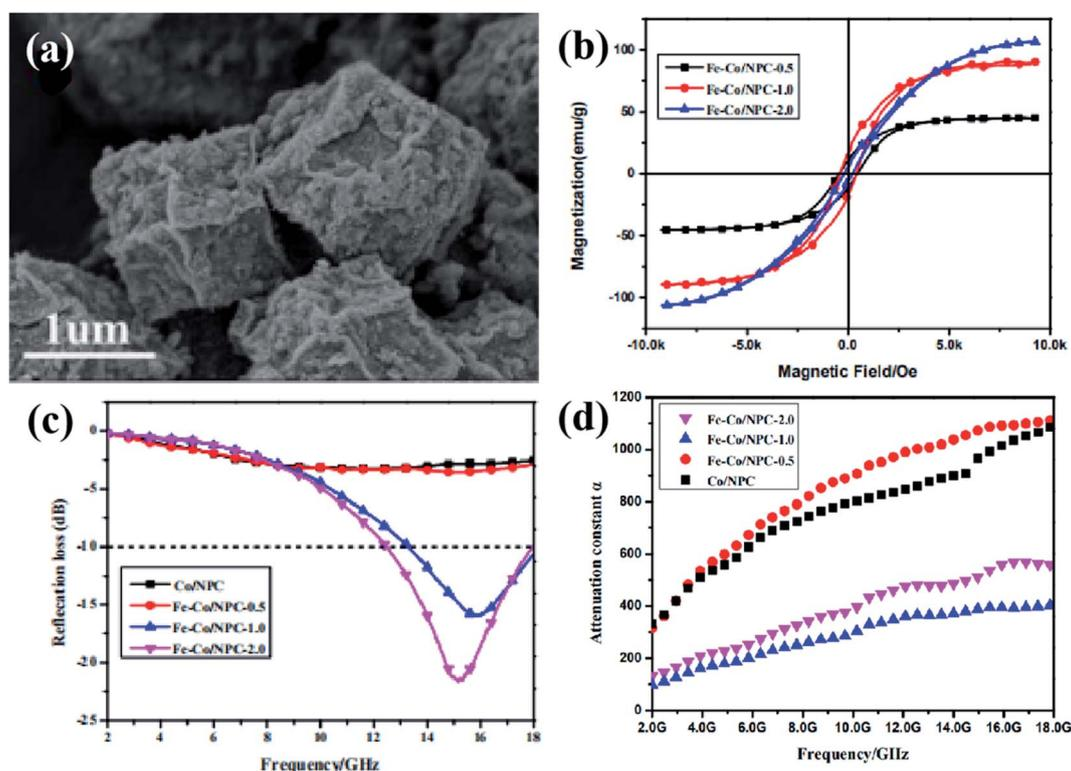
Fig. 7 SEM image of Fe-Co/NPC (a), field-dependent magnetization curve of Fe-Co/NPC (b), the RL (c) and attenuation constant (d) of the Co/NPC, Fe-Co/NPC. This figure has been adapted from ref. 14 with permission from Nanoscale, Copyright 2015.
