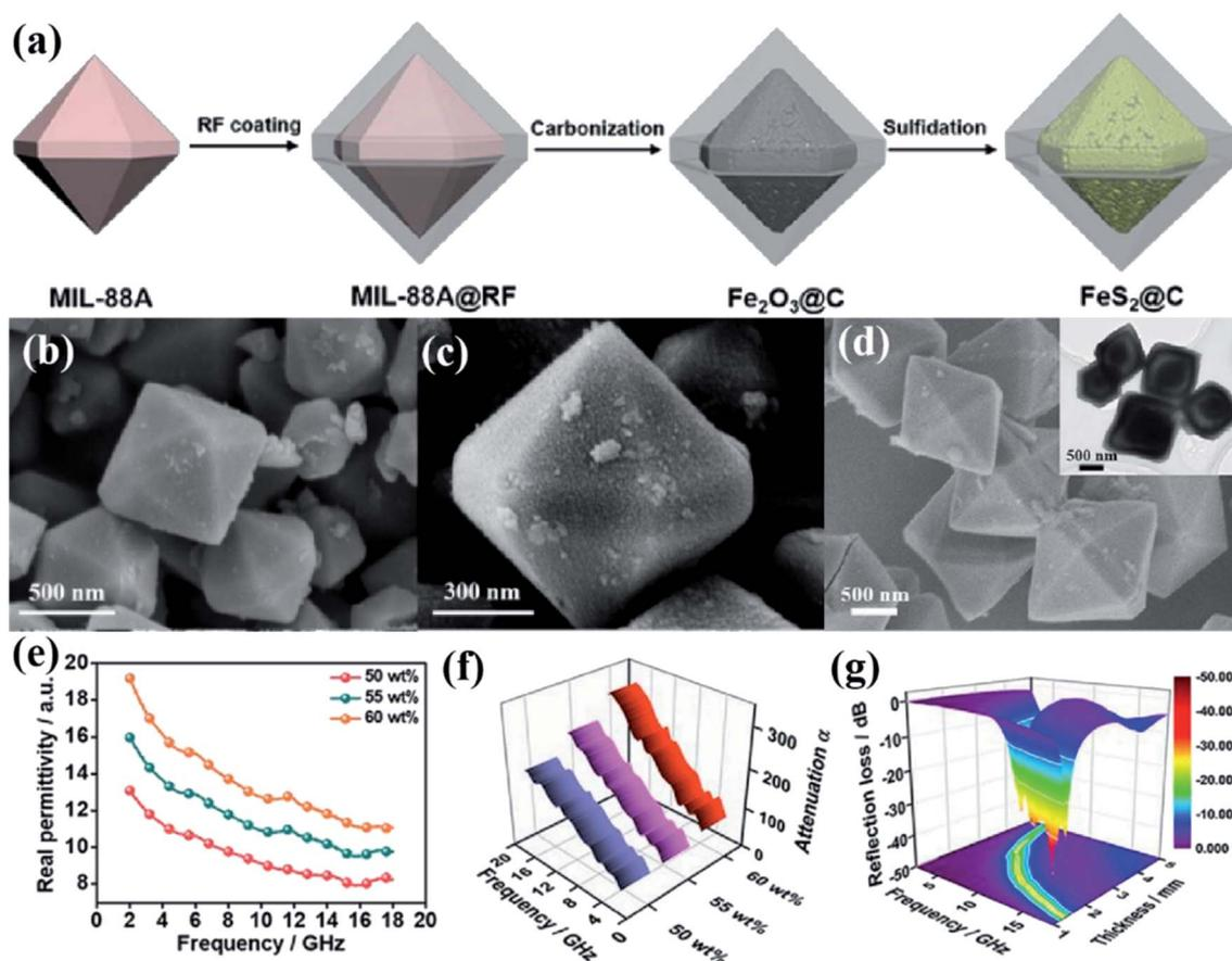
Fig. 9 The schematic formation process of  $\text{FeS}_2\text{/C}$  composites (a), SEM images of Fe-MOF (b),  $\text{Fe}_3\text{O}_4\text{/C}$  (c), SEM and TEM images of  $\text{FeS}_2\text{/C}$  (d), the real permittivity (e), attenuation constant (f) and the RL of  $\text{FeS}_2\text{/C}$  composites (g). This figure has been reproduced from ref. 16 with permission from Nano Letters, Copyright 2020.
