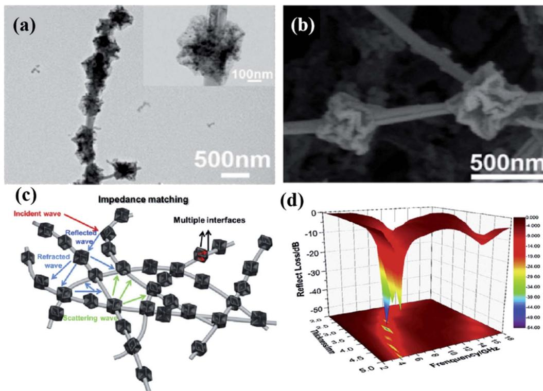
Fig. 10 TEM (a) and SEM (b) images, schematic diagram of microwave absorption mechanisms (c) and the RL (d) of CNFs@Co/CoO composites. This figure has been reproduced from ref. 140 with permission from Journal of Alloys and Compound, Copyright 2018.
