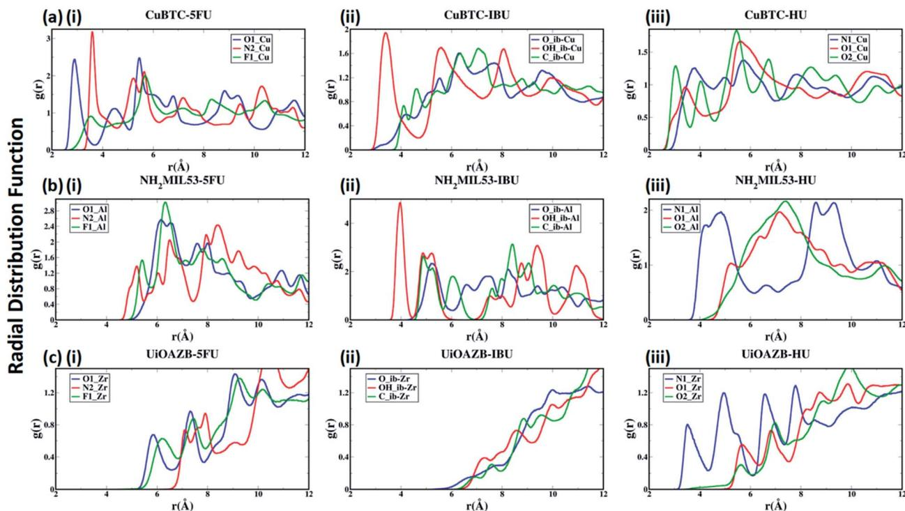
Fig. 2 Radial distribution functional (RDF) analysis of selected atoms of drugs (i) 5-FU, (ii) IBU and (iii) HU with unsaturated metal sites of (a) HKUST-1, (b) NH<sub>2</sub>-MIL-53 and (c) UiO-AZB.
