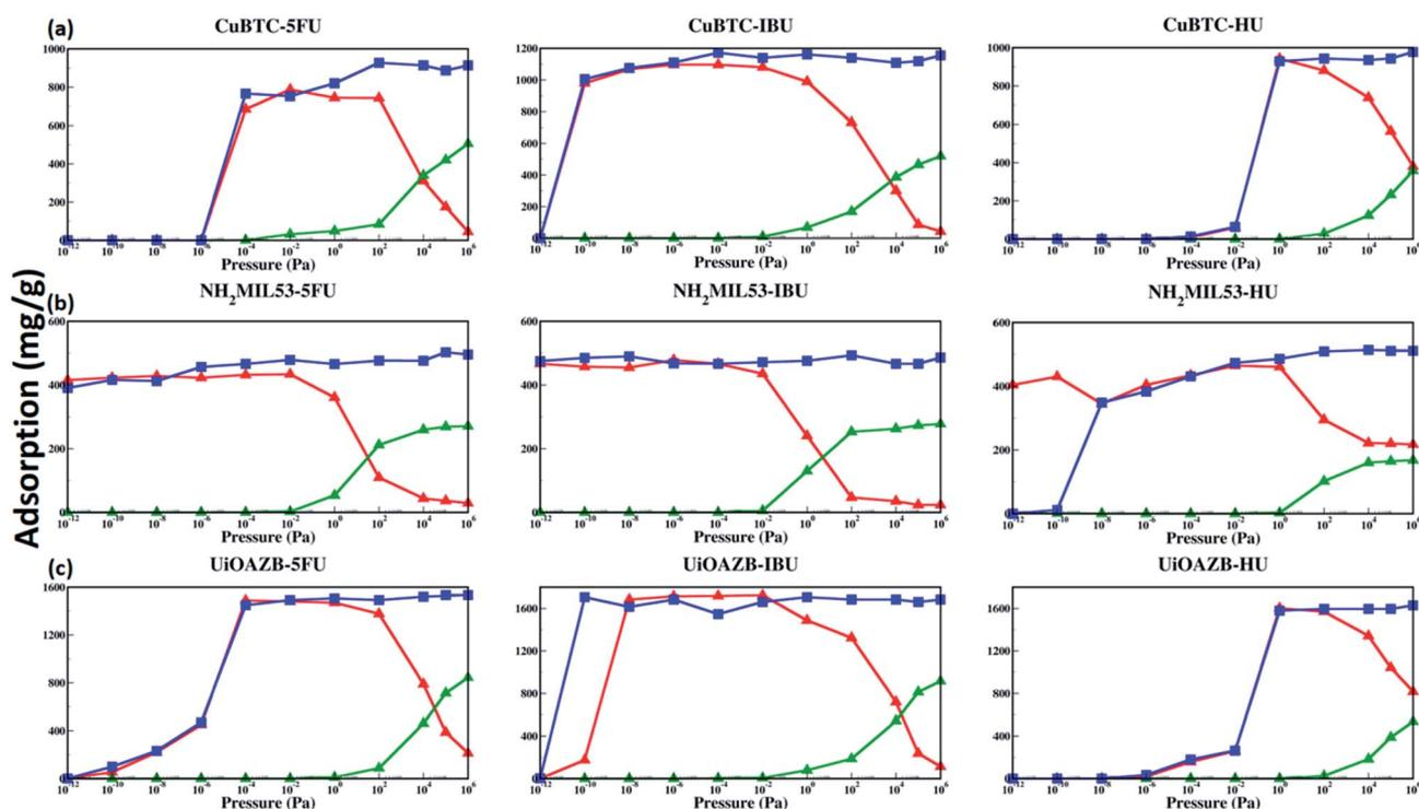
Fig. 3 Adsorption isotherm of the drugs in the presence (red triangles) and absence (blue squares) of ethanol in (a) HKUST-1, (b) NH<sub>2</sub>-MIL-53 and (c) UiO-AZB. Adsorption of ethanol is also shown (green triangles).
