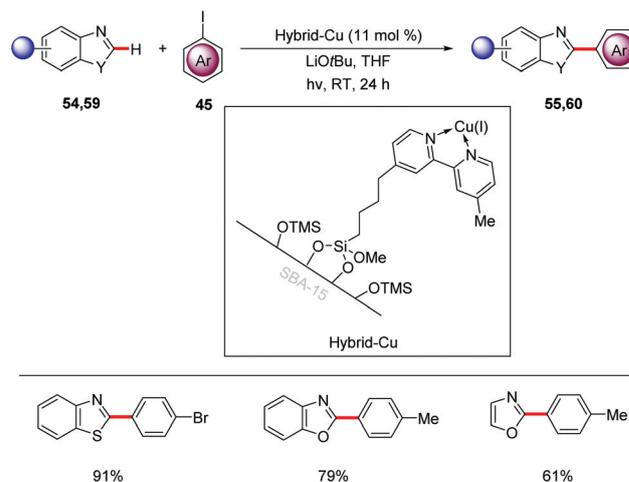
Scheme 20 Heterogeneous copper-catalyzed photo-induced C–H arylation.
