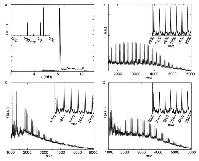
Fig. 3 Mass spectrometry analysis of prepared PUIs. (A) HPLC-MS trace of sPUI-S1; the inset is the MS-spectrum of the dominant peaks at about t = 8.2 minutes showing [M + H $^+$ ], [M + Na $^+$ ] and [M-Boc + H $^+$ ] adducts. (B-D) MALDI-TOF-MS spectra of PUI-A1 (B), PUI-S2 (C) and PUI-A2 (D). Matrix: CHCA with added KAc. Mode: positive linear. Insets are zoom-ins. Enlarged pictures with details on the recorded masses in the arrays are collected in the ESI.
