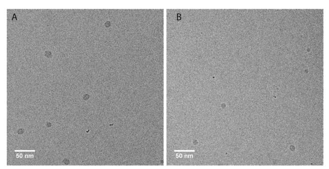
Fig. 4 Cryo-TEM micrographs of PUI-A2 (A) and PUI-S2 (B) after vitrification from aqueous 0.1 M TEA solutions. The grey spots are the micelles vitrified in the ice layer, while the smaller black spots are ice-crystal artefacts at the surface. Concentration: approximately 2.5 mg mL $^{-1}$ . Magnification: 48 000. The ESI contains additional cryo-TEM micrographs with ESI.†
