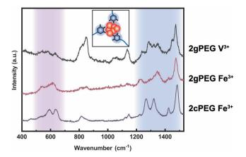
Fig. 5 Raman characterization of 2gPEG hydrogels. Resonance Raman spectra of 2gPEG crosslinked with V3+ and Fe3+, and 2cPEG crosslinked with Fe<sup>3+</sup>. The peaks between 500 and 680 cm<sup>-1</sup> are attributed to the catechol-Fe<sup>3+</sup> coordination or pyrogallol-Fe<sup>3+</sup> coordination, while the peaks between 1230 and 1500 cm<sup>-1</sup> are due to the carbon ring vibration
