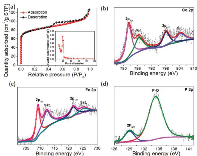
Fig. 5 (a) Nitrogen adsorption–desorption isotherm (the inset shows the pore size distribution curve) for  $\text{CoP}_2/\text{Fe-CoP}_2$  YSBs. (b) High-resolution XPS spectra of  $\text{Co } 2\text{p}$ , (c)  $\text{Fe } 2\text{p}$  and (d)  $\text{P } 2\text{p}$  for  $\text{CoP}_2/\text{Fe-CoP}_2$  YSBs.
