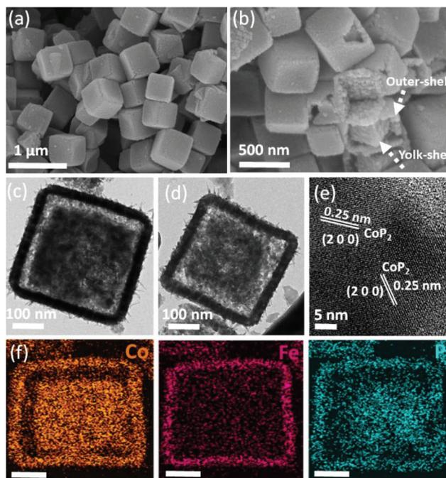
Fig. 4 (a and b) SEM and (c and d) TEM images of  $\text{CoP}_2/\text{Fe-CoP}_2$  YSBs. (e) Corresponding HR-TEM image and (f) STEM mapping images (scale bar: 100 nm).
