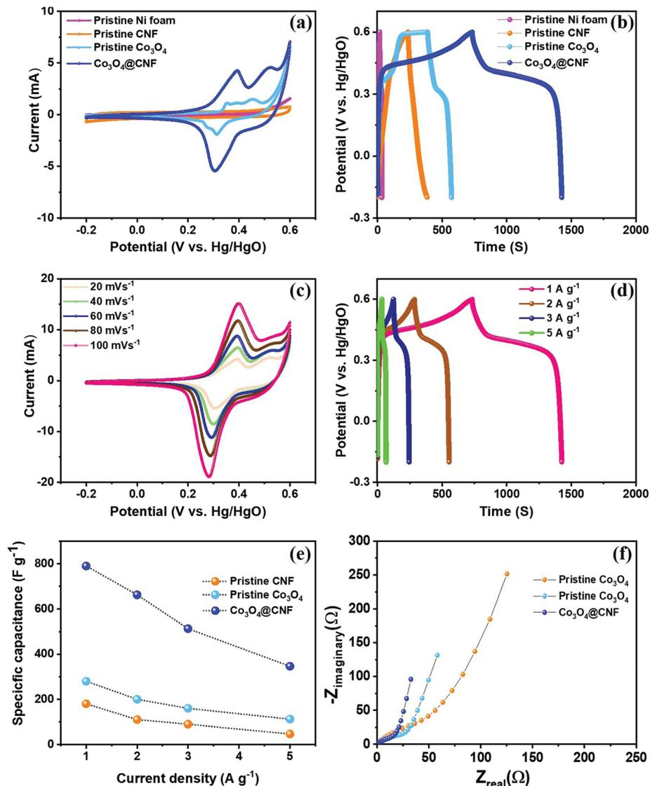
**Fig. 5** Comparison of three electrode electrochemical measurements for the pristine Co<sub>3</sub>O<sub>4</sub> nanoparticles, pristine CNF and 1D Co<sub>3</sub>O<sub>4</sub>@CNF: (a) CV curve at 20 mV s<sup>-1</sup> of scan rate, (b) GCD curve of 1 A g<sup>-1</sup> of current density, (c) and (d) CV and GCD curves at various scan rates and current densities, (e) specific capacitance and (f) EIS measurement.
