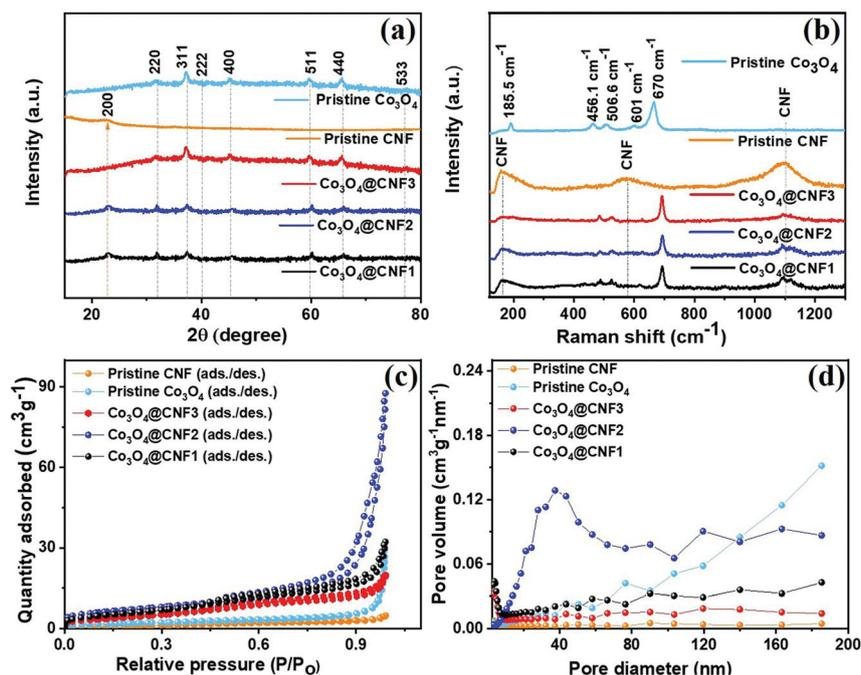
Fig. 2 (a) XRD pattern, (b) Raman spectra, (c) and (d) adsorption–desorption isotherm and BJH curves of the CNF,  $\text{Co}_3\text{O}_4$  nanoparticles, 1D  $\text{Co}_3\text{O}_4$ @CNF3, 1D  $\text{Co}_3\text{O}_4$ @CNF2 and 1D  $\text{Co}_3\text{O}_4$ @CNF1 hybrids.
