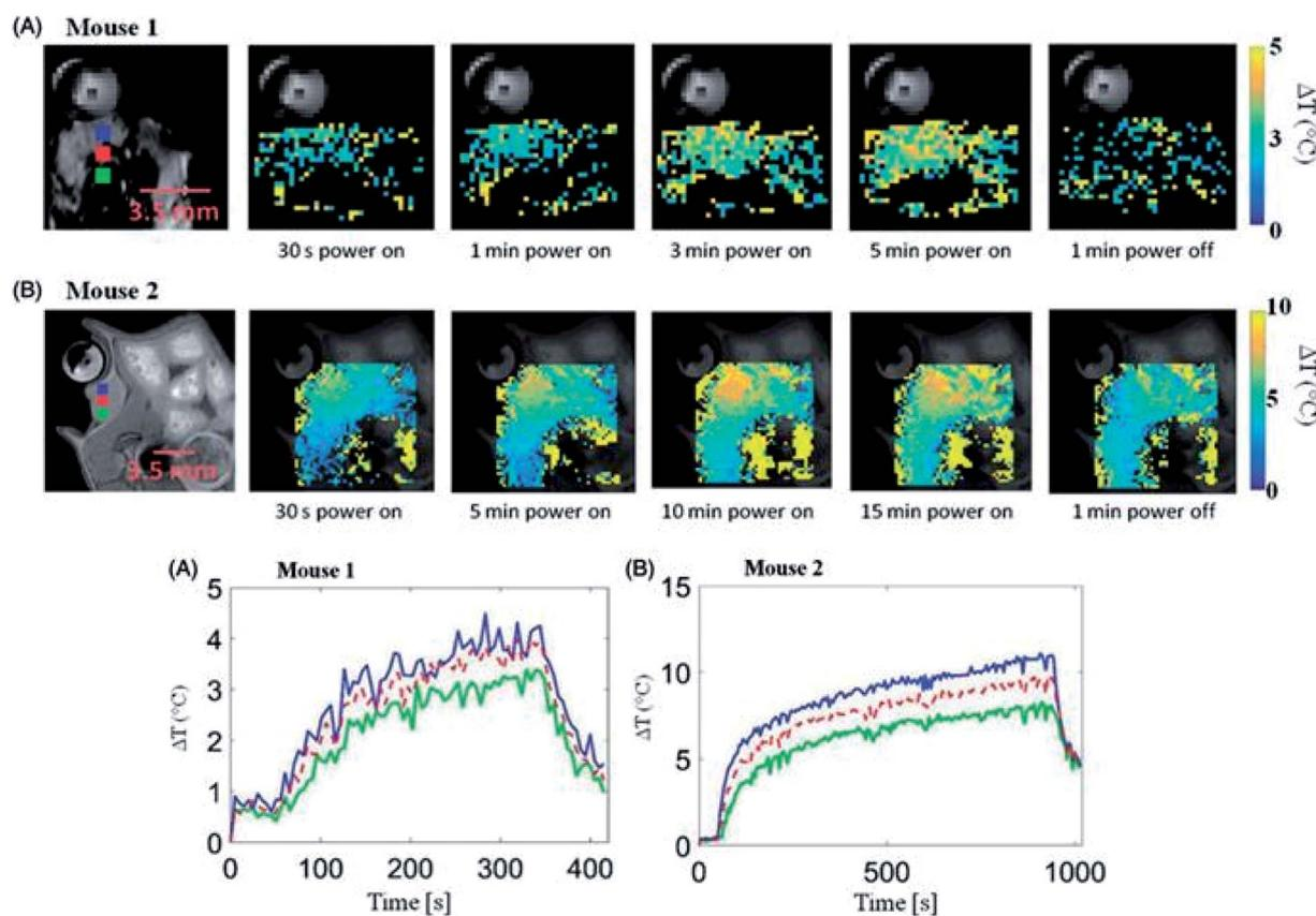
Fig. 6 (Upper panel) Transient evolution of spatial temperature profiles during and microwave exposure *in vivo* with 20 W input power. (Lower panel) *In vivo* transient temperature profiles within subcutaneous tumours during microwave exposure. Reproduced from ref. 85 with permission from the publisher-Taylor & Francis Ltd, <http://www.tandfonline.com>.
