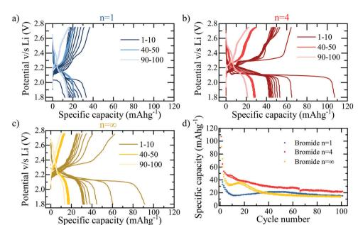
Fig. 4 Galvanostatic cycling of the first insertion mechanism in the reduced potential window of 2.8-1.8 V at a current density of 30 mA g<sup>-1</sup> for the layered perovskites  $(BA)_2(MA)_{n-1}Pb_nBr_{3n+1}$  probing the lithium insertion process stability in (a) n=1 (b) n=4 and (c) the bulk equivalent MAPbBr<sub>3</sub> perovskite structures. (d) Specific capacity of the layered bromide series for the first 100 galvanostatic charge-discharge cycles.
