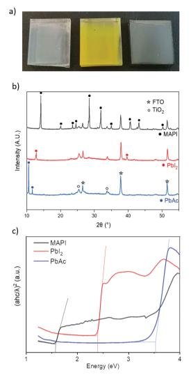
Fig. 3 (a) Photographs of three films removed at different stages of the AACVD deposition (substrate size 12 mm  $\times$  12 mm). Left: Film after first step. Centre: Film halfway through MAI aerosol exposure. Right: Completed MAPI film (b) XRD patterns correspond to initial PbAc<sub>2</sub> film, PbI<sub>2</sub> intermediary and final MAPI film (c) Tauc plots of the three films calculated from absorption data.
