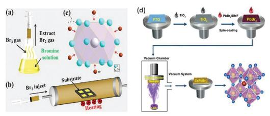
Fig. 8 (a)  $Br_2$  vapor extraction from a bottle of Br water; (b) schematics of the  $Br_2$  vapor-assisted CVD process; and (c) crystal structure. Reproduced with permission ref. 121. Copyright 2018, Elsevier Ltd. (d) Illustration of the evaporation-assisted solution method (EAS) to prepare a  $CsPbBr_3$  thin film. Reproduced with permission ref. 120. Copyright 2019, American Chemical Society.
