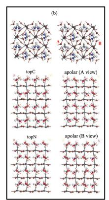
Fig. 2 Top and side views of (a) cubic and (b) tetragonal MAPbI $_3$ (001) surfaces with MAI terminations for topC, topN and apolar geometries. Two different side views (from A and B sides) of the tetragonal MAPbI $_3$ (001) surface are shown for clarity. H, C, N, I, and Pb atoms are represented by the white, light grey, blue, brown, and dark grey spheres, respectively. Red arrow represents the molecular dipole of a MA cation with the NH $_3$  group as the arrow head.
