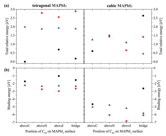
Fig. 5 (a) Total DFT-D and (b) binding energies of a MAPbl $_3/C_{60}$  heterojunction relative to the topC-aboveC configuration. Orientations of the MA cation with respect to the (001) surface are: topC (black), topN (red) and apolar (blue).
