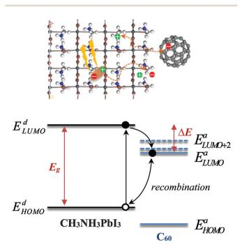
Fig. 1 Schematic illustration of the energy-level diagram for the MAPbI<sub>3</sub> and  $C_{60}$  in the hybrid perovskite/fullerene heterojunction.  $E_q$  is the energy gap of MAPbI<sub>3</sub> and  $\Delta E$  is the dissociation energy of the electron-hole pairs. The three-fold degenerate LUMO of  $C_{60}$  fullerene has three energy levels from the LUMO to LUMO+2.
