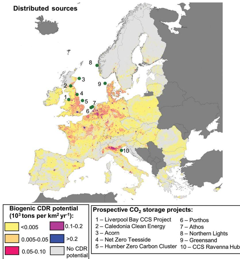
Fig. 3 Geospatial distribution of biogenic carbon dioxide removal potential from distributed sources of biogenic CO<sub>2</sub> in Europe. Distributed sources of biogenic CO<sub>2</sub> are livestock manure, household organic food waste, and crop residues. The figure shows location and name of ten prospective carbon storage sites that are planned or in start-up phase in Europe.
