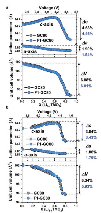
Fig. 5 Unit cell contraction of GC80 and F1-GC80 cathodes during delithiation. The lattice parameter and unit cell volume change for GC80 and F-GC80 cathodes by in situ XRD analysis; (a) first cycle and (b) after 2000 cycles.
