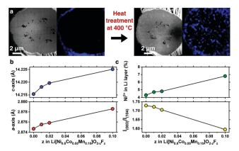
Fig. 1 Structural details of the F-doped GC80 cathodes. (a) EDS mapping of F Ka emission for a cross-section of the F-doped GC80 before (left-hand side) and after the heat treatment (right-hand side). (b) Calculated a- and c-axis lattice parameters with increasing amount of F doping. (c) Cation mixing of Ni<sup>2+</sup> in the Li layer and intensity ratio of the (003) peak to (104) peak as a function of the F concentration.
