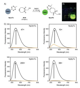
Fig. 2 (A) Schematic of fluorogenic reaction between naphthalimide (Naph) tetrazines after reaction with BCN to form pyridazine products in situ. (B) Photograph of vials of Np6mTz (left) and Np6mPz (right) in dichloromethane, under 365 nm light. (C) Emission spectra of 5 µM solutions of naphthalimide tetrazines (orange) and the corresponding pyridazine products (black). Numbers indicate the fold turn-on as determined by integration of the spectra.
