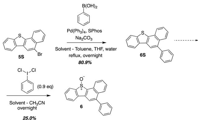
Scheme 3 Synthesis of **6** which represents the core structure of **2** and **3**.
