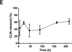
Fig. 2 Representative SEM images of PLA-NPs (A and C) and CLIN-PLA-NPs (B and D) at low and high magnification. Scale bars: 3  $\mu$ m (top) and 1  $\mu$ m (bottom). Profile of clindamycin release from the nanoparticles in PBS at 37 °C (N=3) (E).
