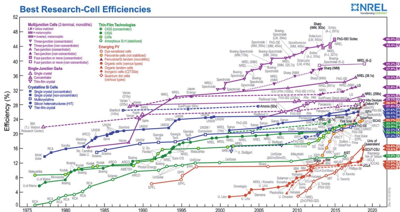
Fig. 8 2019 plot of highest-recorded photovoltaic efficiency by year of various photovoltaic devices classified by technology (colours). Prepared by the National Renewable Energy Laboratory (NREL, <http://www.nrel.gov>).
