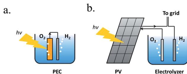
**Fig. 1** (a) Scheme of a PEC system immersed in the electrolyte, where one of the electrodes is photoactive. (b) Scheme of a photovoltaic panel connected to an electrolyzer with the option to give or take current to the electrical grid.
