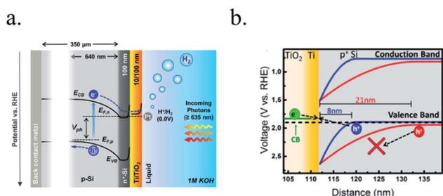
Fig. 25 Metallic thin Ti films on degenerately-doped silicon assuring ohmic contacts in (a) a photocathode (reprinted with permission from *Sol. Energy Mater. Sol. Cells*, 2016, **144**, 758–765). Copyright (2016) Elsevier.<sup>145</sup>) and (b) a photoanode, where holes recombine with electrons from the conduction band of the protective layer (reprinted with permission from *J. Phys. Chem. C*, 2015, **119**, 15019–15027). Copyright (2015) American Chemical Society<sup>252</sup>).
