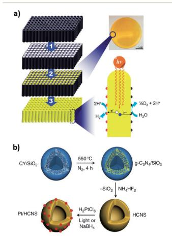
Fig. 9 (a) Synthesis of CN nanorods confined in an AAO template. Reproduced from ref. 336. Copyright (2011) American Chemical Society. (b) Synthesis of CN nanospheres utilizing silica nanoparticles. Reproduced with permission from ref. 338, copyright (2012) Nature publishing group.
