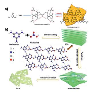
Fig. 12 Synthesis of a supramolecular complex based on melamine and nitric acid and its conversion into porous CN nanosheets. (a) Reproduced from ref. 425, copyright (2019) Materials Research Society. (b) Reproduced from ref. 434, copyright (2019) Elsevier publishing group.
