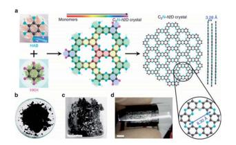
Fig. 2 Schematic representation of the synthesis of a C<sub>2</sub>N material (a), and its corresponding digital images as prepared (b), solution cast over SiO<sub>2</sub> after condensation at high temperatures (c) and in a film over a PET substrate (d). Reproduced with permission from ref. 75, copyright (2015) Nature publishing group
