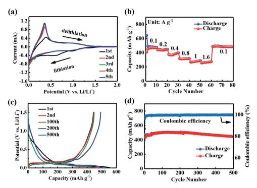
Fig. 2 (a) CV curves at a scan rate of  $0.1 \text{ mV s}^{-1}$ , (b) rate performance at varied currents, (c) charge/discharge profiles and (d) long cycling performance at  $100 \text{ mA g}^{-1}$  of the Si/C electrode.
