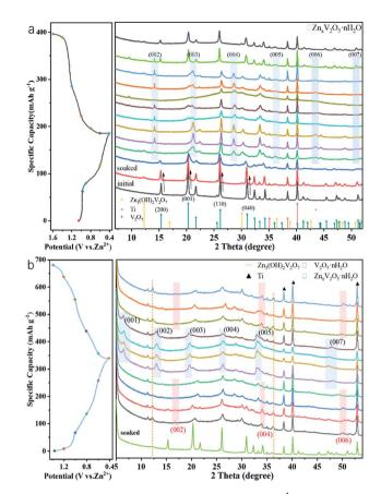
Fig. 5 Typical discharge–charge curve at 0.05 A  $\rm g^{-1}$  and ex situ XRD patterns of the  $\rm V_2O_5$ -YS cathode at different voltages vs. Zn<sup>2+</sup>/Zn (a) in the first cycle (b) and in the 11th cycle.
