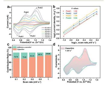
Fig. 3 (a) CV curves of the  $V_2O_5$ -YS cathode at various scan rates, (b) plots of log(peak current) versus log(scan rate) based on the four main peaks, (c) ratio of capacitive and diffusion-controlled capacities at multiple scan rates, and (d) CV curve displaying the capacitive contribution (shadow area) to the total current at 1.0 mV  $s^{-1}$ .
