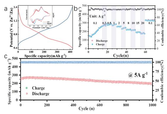
Fig. 2 Electrochemical performance of the  $Zn/V_2O_5$ -YS battery: (a) galvanostatic discharge/charge profiles at a current density of 0.1 A  $q^{-1}$ (inset: the corresponding dQ/dV curve (blue) and CV curves (red)); (b) rate capability; (c) long cycling performance at 5.0 A  $g^{-1}$
