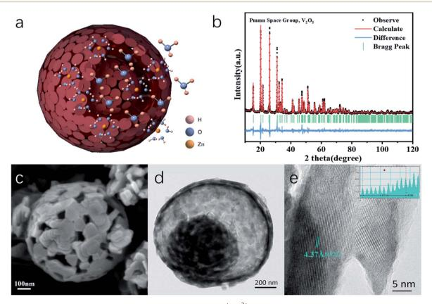
Fig. 1 (a) Schematic of the as-prepared  $V_2O_5$ -YS microspheres with the  $H^+/Zn^{2+}$  co-insertion process. (b) Rietveld refinement results of the Xray diffraction (XRD) pattern, (c) SEM image, (d) TEM image, and (e) HRTEM image of the V<sub>2</sub>O<sub>5</sub>-YS microspheres.
