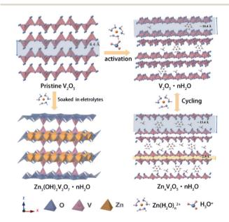
Scheme 1 Schematic illustration of the energy storage mechanism during activation and cycling processes.
