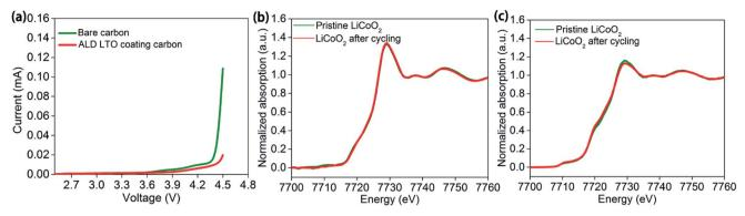
Fig. 5 (a) Comparison of the linear sweep voltammogram of the Li/SPE/PEO-carbon composite cell and Li/SPE/PEO-LTO@carbon composite cell (scan rate = 0.3 mV s<sup>-1</sup>, from OCV to 4.5 V vs. Li/Li<sup>+</sup>). Comparison of the XAS Co K-edge spectra of unprotected LiCoO<sub>2</sub> before and after 5 cycles of charge/discharge in ASSLBs in the discharge state in terms of (b) TEY mode and (c) FLY mode.
