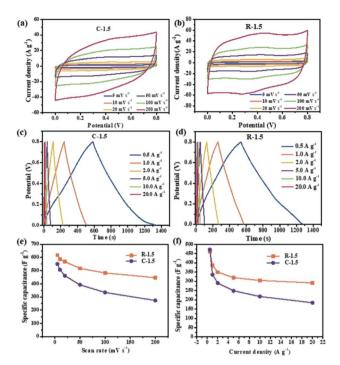
Fig. 6 CV curves of C-1.5 (a) and R-1.5 (b) at different scan rates; GCD curves of C-1.5 (c) and R-1.5 (d) at different current densities; specific capacitances calculated from CV curves (e) and GCD curves (f).
