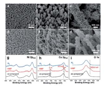
Fig. 6 SEM images of  $Cu_xS@Ni_{0.75}Co_{0.25}O_mH_n$  after catalyzing long-term HMF oxidation (a–c) and HER (d–f). Ni  $2p_{3/2}$  (g), Co  $2p_{3/2}$  (h) and O 1s (i) XPS spectra of  $Cu_xS@Ni_{0.75}Co_{0.25}O_mH_n$  after catalyzing long-term HMF oxidation (labeled as 'HMF') and hydrogen evolution reaction (labeled as 'H<sub>2</sub>').
