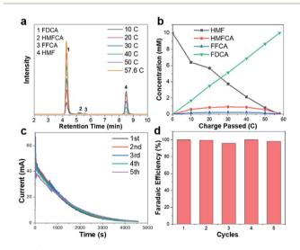
Fig. 3 (a) HPLC chromatogram traces of electrolyte during the electrochemical oxidation of HMF catalyzed by  $Cu_xS@Ni_{0.75}Co_{0.25}O_mH_n$  at 1.32 V vs. RHE. (b) Concentration profiles of oxidation products with increasing charge. (c) Current–time curves and (d) faradaic efficiency towards FDCA in 5 successive runs.
