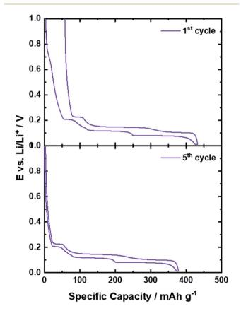
Fig. 5 Comparison of the potential profile of graphite half-cells for the  $1^{st}$  (upper panel) and  $5^{th}$  (lower panel) dis-/charge cycle.
