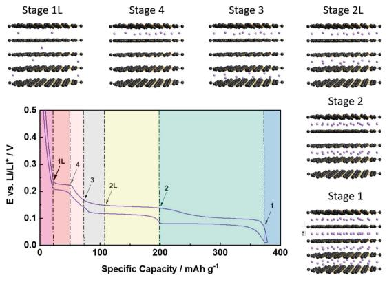
Fig. 4 Illustration of the staging mechanism for the electrochemical de-/intercalation of lithium cations (purple spheres) into graphite. The given representative potential profile refers to the 2<sup>nd</sup> dis-/charge cycle in half-cell configuration, i.e., vs. metallic lithium as counter electrode.
