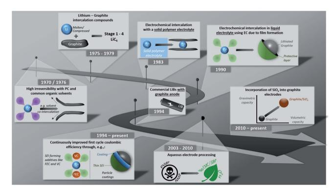
Fig. 1 Illustrative summary of major milestones towards and upon the development of graphite negative electrodes for lithium-ion batteries.
