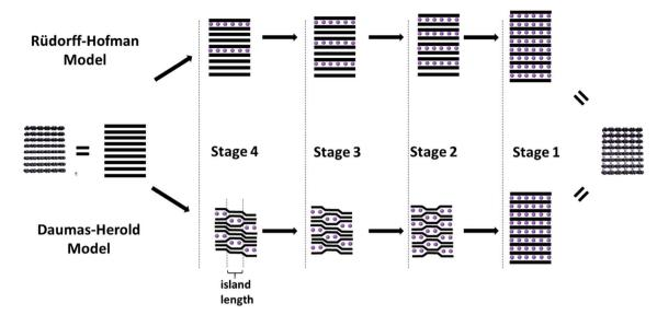
Fig. 3 Schematic illustration of the intercalation mechanism of secondary species (i.e., the intercalant; purple spheres) into the layered graphite structure (illustrated by the black lines) according to the model of Rüdorff and Hofmann (upper path) and Daumas and Herold (lower path; figure partially redrawn from ref. 69)
