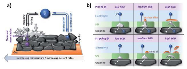
Fig. 8 (a) Schematic illustration of lithium plating/stripping on graphite electrodes in competition with the de-/intercalation of lithium cations into graphite depending on the applied current and temperature (figure redrawn from ref. 211). (b) The behavior of plated lithium metal on top of a graphite electrode as a function of the 'state of charge' (SOC) and 'state of discharge' (SOD) upon plating and stripping, respectively (figure redrawn from ref. 215).
