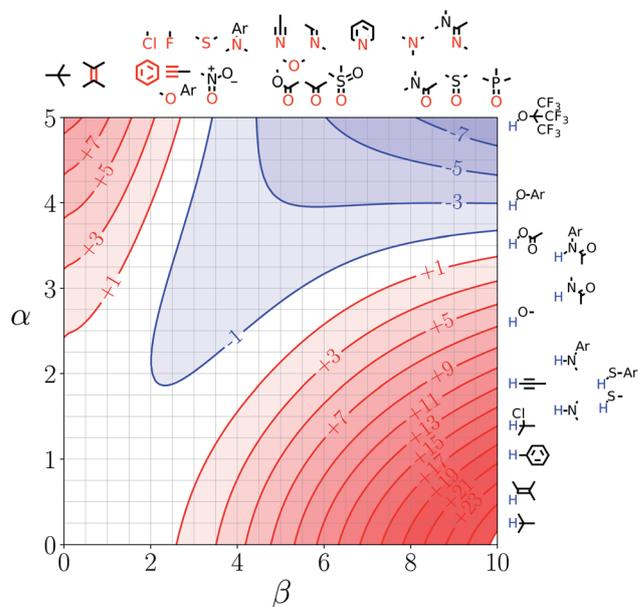
Fig. 7 FGIP for the interaction of two solutes in formic acid at 298 K ( $\Delta\Delta G_{\text{FGI}}$  in  $\text{kJ mol}^{-1}$ ). The solute–solute interactions in the blue region, and unfavourable in the red region.
