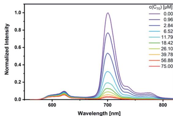
Fig. 6 Steady-state fluorescence spectra of *syn*-SubPc 1 ( $1.5 \times 10^{-6}$  M) after 440 nm excitation in toluene with increasing amount of C<sub>70</sub> (0–75 μM).
