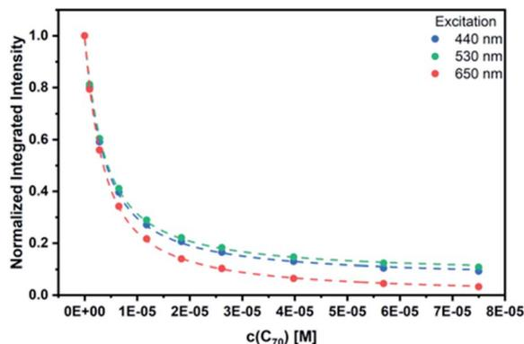
Fig. 7 Binding isotherms obtained during the titration of *syn*-SubPc 1 with C<sub>70</sub> by means of steady-state fluorescence spectroscopy.
