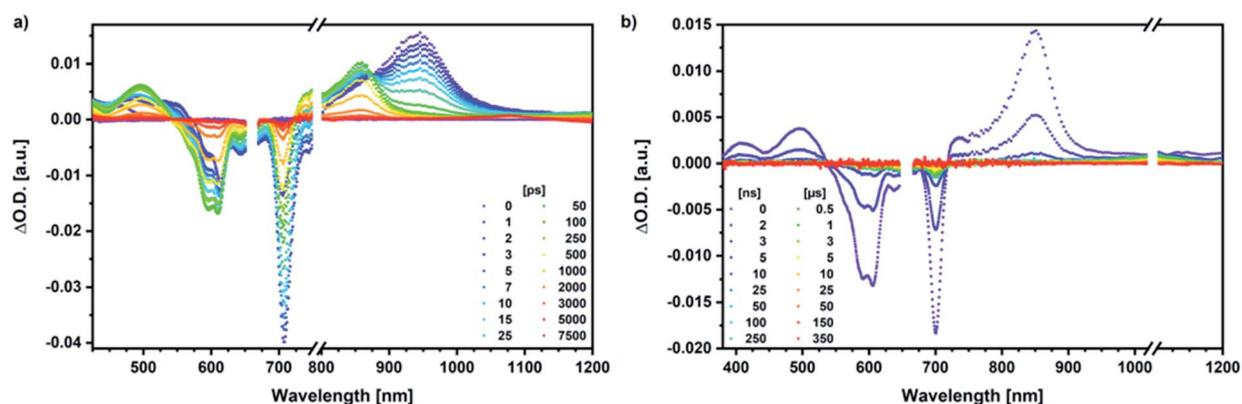
Fig. 9 (a) Femtosecond differential absorption spectra of *syn*-SubPc 1 ( $1.5 \times 10^{-5}$  M) in argon purged chlorobenzene at delay times between 0 and 7500 ps after 656 nm laser excitation (200 nJ) at room temperature. (b) Nanosecond differential absorption spectra of *syn*-SubPc 1 ( $1.5 \times 10^{-5}$  M) in argon purged chlorobenzene at delay times between 0 and 350  $\mu$ s after 656 nm laser excitation (450 nJ) at room temperature.
