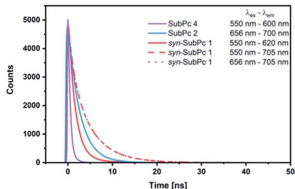
Fig. 8 Fits of fluorescence decays obtained by the time correlated single photon counting method of monomer-SubPc 4 ( $1.5 \times 10^{-6}$  M), dimer-SubPc 2 ( $1.5 \times 10^{-6}$  M), and *syn*-SubPc 1 ( $1.5 \times 10^{-6}$  M) in argon purged toluene. The excitation and emission wavelengths were as given in the legend.
