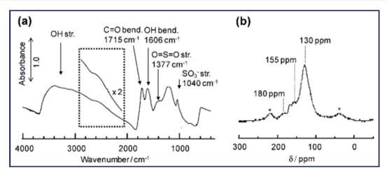
Fig. 29 FT-IR (a) and <sup>13</sup>C MAS NMR (b) spectra for the sulfonated carbon catalyst originated from cellulose. Reproduced from ref. 368.
