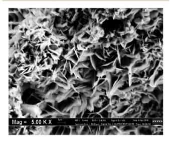
Fig. 10  $\,$  SEM image of Mg–Al HT calcined at 850  $^{\circ}\text{C}.$  Reproduced from ref. 140.
