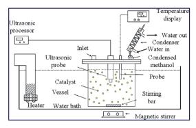
Fig. 3 Schematic portrayal of experimental set up for the ultrasonicassisted transesterification reaction. Reproduced from ref. 86.
