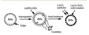
Fig. 11 Proposed model for the solid-state reaction on the catalyst surface. Reproduced from ref. 145
