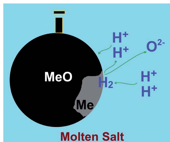
Fig. 6 Hydrogen cations present in molten salts can be reduced on cathodically polarised metal oxides to form water and the corresponding metal. The dissolution of produced water in the molten salt leads to the regeneration of hydrogen cations to precede the reduction process.
