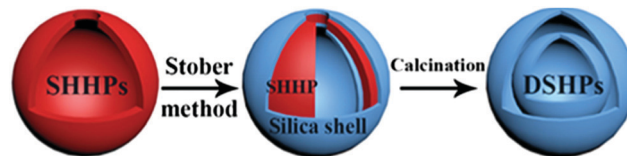
Fig. 14 Schematic of the preparation process of DSHPs. Reprinted from ref. 54 with kind permission.
