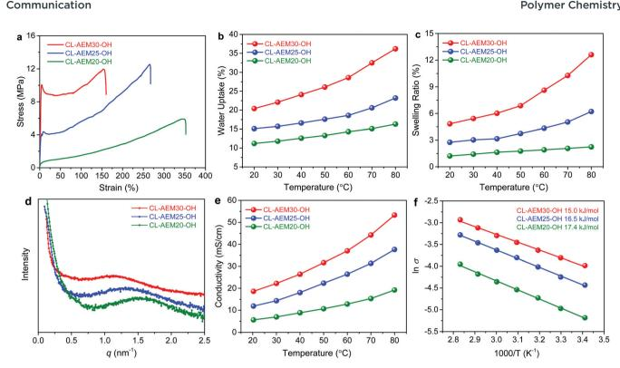
Fig. 1 Crosslinked metallo-polyelectrolyte membranes: (a) stress-strain curves; (b) water uptake; (c) swelling ratios; (d) SAXS profiles; (e) hydroxide conductivity as a function of temperature under fully hydrated conditions; and (f) Arrhenius plots.
