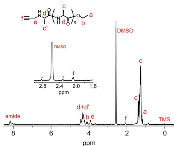
**Fig. 3**  $^1\text{H}$  NMR spectrum of poly(L-alanine) with an alkyne moiety at the N-terminus synthesized via papain-catalyzed polymerization at the Ala-OEt/2 feed ratio of 1/0.2. Asterisk shows spinning side bands of solvent peak.
