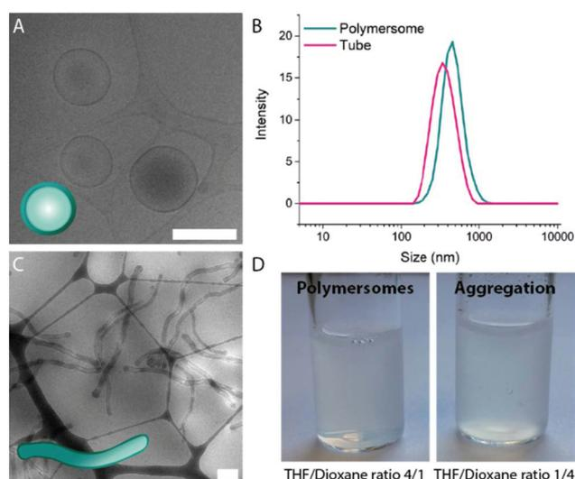
**Fig. 2** Cryo-TEM images of spherical polymersomes (A) and tubular polymersomes (C). (B) Hydrodynamic size of polymersomes and tubes measured by DLS. Please note the difference in size in polymersomes and tubes which is a result of the volume reduction following the shape transformation process. (D) Formation of polymersomes (left) and aggregation (right) with varying THF:dioxane ratio. Scale bars are 500 nm.
