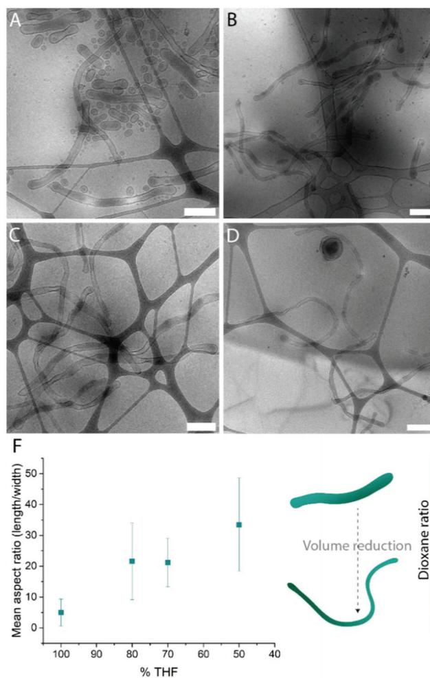
**Fig. 3** Cryo-TEM images of tubes formed with THF:dioxane ratio (v/v%) (A) 100 : 0, (B) 80 : 20, (C) 70 : 30 and (D) 50 : 50. Mean aspect ratio measured from image analysis (F). Scale bars are 500 nm.
