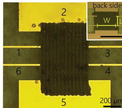
**Fig. 1** Optical micrograph showing a representative graphene Hall bar fabricated on fused quartz with 40 print passes. In the inset, the back-side of the same device is presented. The scale bar in the inset corresponds to  $500 \text{ } \mu\text{m}$ .
