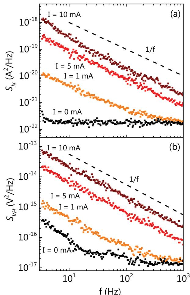
Fig. 6 log–log plot of (a)  $S_{I_x}$  and (b)  $S_{V_H}$ , as a function of  $f$  for a device fabricated on fused quartz with 40 print passes and for different bias currents. As a reference, the  $1/f$  slope is shown as a dotted line.
