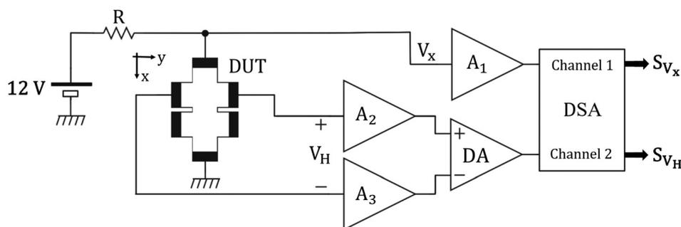
Fig. 5 Schematic diagram of the setup used for low-frequency noise characterization.  $A_1$ ,  $A_2$ , and  $A_3$  are single-ended amplifiers. DA is a differential amplifier and DSA is a dynamic signal analyzer.
