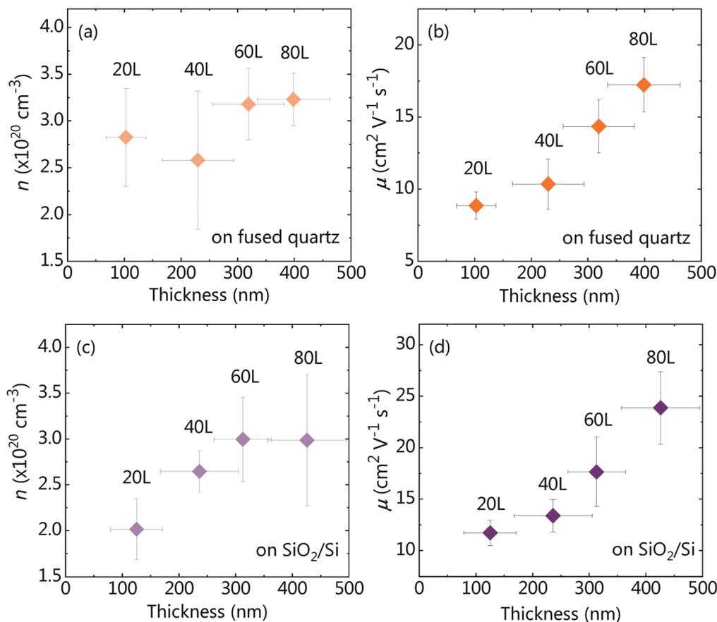
**Fig. 3** Average values of  $n$  and  $\mu$  determined from Hall bar analysis for the devices printed on fused quartz [(a) and (b)] and on  $\text{SiO}_2/\text{Si}$  [(c) and (d)], with 20, 40, 60 and 80 print passes. The error bars on the film thickness and on the average values of  $n$  and  $\mu$  represent the mean RMS roughness and the standard error, respectively.
