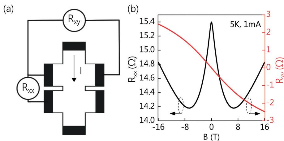
**Fig. 4** (a) Magnetoconductance measurement scheme and (b) magnetoconductance spectra taken at 5 K for a device fabricated on fused quartz with 80 print passes, showing the standard weak-localization behavior.
