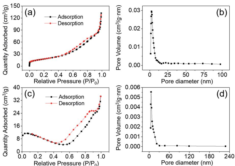
Fig. 7 Nitrogen adsorption–desorption isotherms and the corresponding BJH pore-size distribution plots of (a and b) the  $\text{MgCo}_2\text{O}_4$  NFs and (c and d) the  $\text{MgCo}_2\text{O}_4$  NCs, respectively.
