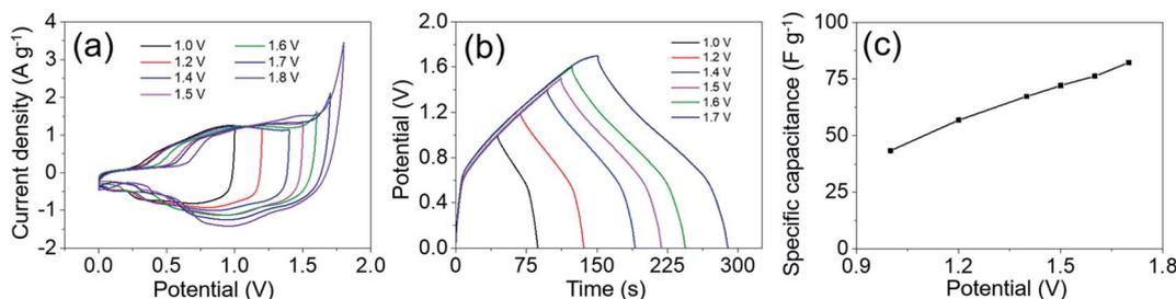
Fig. 11 (a) CV curves of the  $\text{MgCo}_2\text{O}_4$  NFs//AC ASC measured over different voltage windows at a scan rate of 10  $\text{mV s}^{-1}$ , (b) GCD curves of the  $\text{MgCo}_2\text{O}_4$  NFs//AC ASC measured over different voltage windows at a current density of 1  $\text{A g}^{-1}$ , and (c) specific capacitance as a function of voltage windows.
