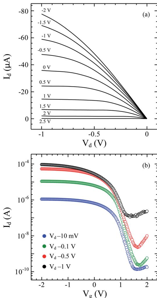
Fig. 2 (a). Output characteristics ( $I_d$  versus  $V_d$  curve) of the device fabricated from the Ge-core/a-Si shell nanowire with  $V_g = 2$  to  $-2.5$  V in steps of 0.5 V from the top to the bottom. (b) Transfer characteristics ( $I_d$  versus  $V_g$  curve) of the device at  $V_d = -0.01$ ,  $-0.1$ ,  $-0.5$  and  $-1$  V. The gate voltage ( $V_g$ ) was swept from  $-2$  to  $2$  V. The channel length is 800 nm.
