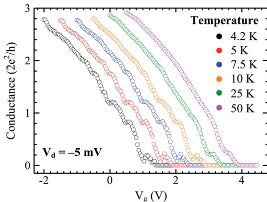
Fig. 9 Conductance versus gate voltage at  $V_d = -5$  mV measured at various temperatures. The x-axis has been shifted to the right for clarity of comparison.
