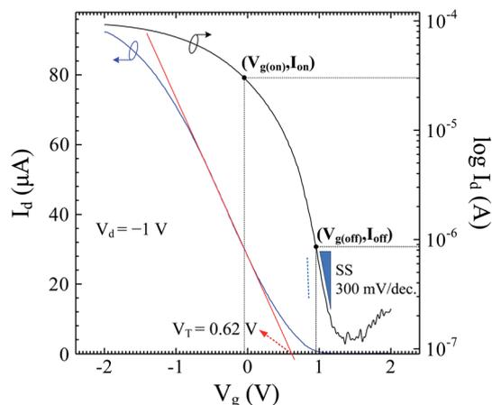
Fig. 3 Transfer characteristics for  $V_d = -1$  V on the linear scale (blue curve) and logarithmic scale (black curve). The red line is the tangent to the maximum slope on the linear scale where the intersection of this line and the x-axis denotes the threshold voltage. The on-off currents were calculated using the metrics defined in ref. 14. The subthreshold slope (SS) is 300 mV per decade. The dashed blue line indicates the physical limit of SS (60 mV per decade at room temperature).
