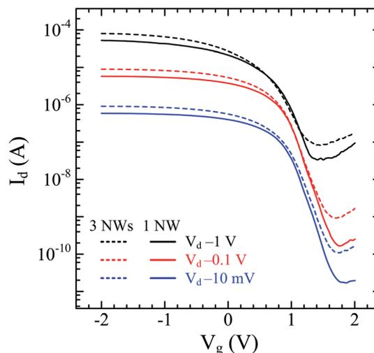
Fig. 5 Transfer characteristics ( $I_d$  versus  $V_g$  curve) of the devices consisting of a single nanowire (solid curves) and three nanowires (dashed curves) at  $V_d$  of  $-0.01$  V,  $-0.1$  V and  $-1$  V. The gate voltage ( $V_g$ ) was swept from  $-2$  to  $2$  V. The channel length is  $1 \mu\text{m}$ .
