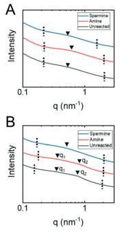
Fig. 4 One-dimensional SAXS traces for P(TFEMA-OEGMA-GMA) copolymer membranes (A) in the dry state and (B) submerged in water. The dashed vertical lines indicate the region of interest and the arrows identify maxima in the broad scattering peaks. The scaling and positions of the traces on the y-axis have been altered to facilitate visualizing the peak positions in reference to q-values.
