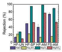
Rejection of salts in a 1 mM feed solution by the unreacted hollow (HF-UN), spermine-functionalized hollow fiber hexamethylene diamine-functionalized hollow fiber (HF-AM), and hexamethylene diamine-functionalized flat sheet (FS-AM) membranes. The cation concentrations in solution were determined using ICP-OES. The error bars represent one standard deviation from n = 2 measurements.
